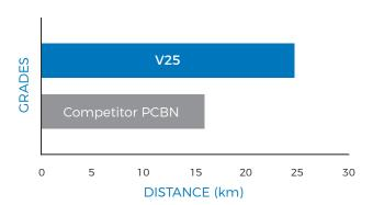
Work Material - 100Cr6, HRc 60-62 Interrupted turning Vc = 160 m/min, ap = 0.2 mm, f = 0.15 mm/rev
